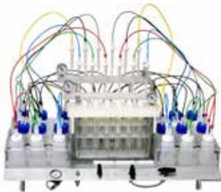
The **EZ-PFC** allows us to perform solid phase extractions for 6 samples in less than 50 minutes achieving high recoveries and excellent precision for all analytes. With the EZPFC we can run multi-cartridge applications for any SPE PFAS/PFOS/PFOA method requiring more than one cartridge. The EZPFC system uses existing EPA Methods 537, 537.1 and other methods for PFAS/PFOS/PFOA extraction and analysis in various matrices.
