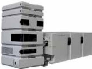
ResinTech uses an **Agilent 6410B LC/MS** for liquid chromatography and mass spectrometry associated with PFAS compounds.
