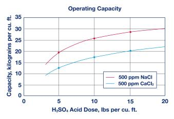
Capacity based on 500 ppm of stated salt (as  $CaCO_3$ ) with 0% alkalinity, 36 in. bed depth, flow rate of 2 to 4 gpm per cu. ft. and >30 min. chemical injection time. Sulfuric acid concentration must be stepwise when calcium concentration exceeds 20% of total cations. No engineering downgrade has been applied.
