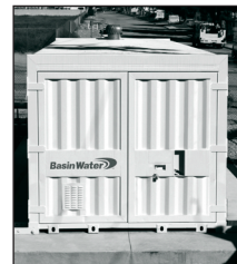
City of Pomona 1000 GPM Nitrate Removal Unit
