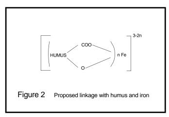
oxidation, are two of the common methods used for removing this form of iron. Many of the carboxylic groups on the humic acid molecules remain ionized, therefore they are free to interact with and be removed successfully by special purpose ion exchange resins, one of which I will discuss later. The presence of heme iron is the reason why most organically fouled anion resins also contain iron. They can also have copper, aluminum, zinc, manganese, etc. which also form complexes with humic acids.
