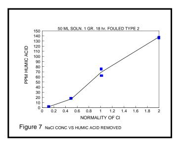
brine is alkaline these groups become fully ionized. In order to keep them ionized and soluble at the high concentrations of regeneration, excess hydroxyl groups are required. Adding caustic to the brine does both.
